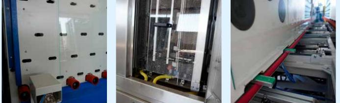
Complete lines for the production of insulating glass, in which different parts of the plant wash, couple and press the double or triple glazing unit in rapid succession.
